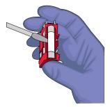
**4.** Replace each failed fuse with a 1.6A, Time-Lag T, 250VAC, 5 × 20-mm Fuse.
