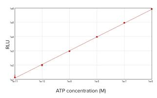
An ATP standard curve spanning five decades was run using the ATPlite 1step Luminescence Assay System (PerkinElmer) on the SpectraMax iD5 reader. Standard concentrations ranged from 1x10-11 M to 1x10-6 M. A wide linear dynamic range ensures accurate assay results across a broad span of sample types. Standards were plotted using a log-log curve fit in SoftMax Pro Software.
